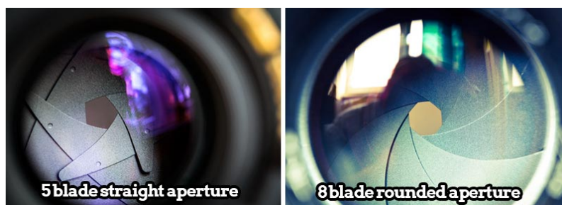
Figure 2.4: Two different apertures, with five straight blades (left) and eight rounded blades (right). Image from https://improvephotography.com/29529/aperture-blades-many-best/
